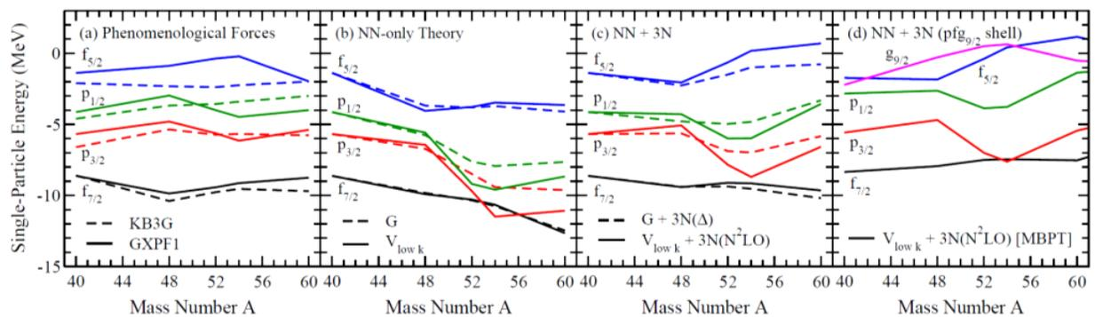
Figure 1: Neutron single-particle energy levels relative to those in  $^{40}\text{Ca}$ , as calculated using (a) phenomenological forces, fit to data; (b) NN-only calculations; (c) NN + 3N calculations, and (d) NN + 3N calculations in an expanded model space. Taken from Reference [Ho11].
