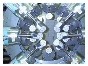
ClassicSeGA: Note that this photo only shows 6 detectors in the forward ring. The forward ring can accommodate up to 8 detectors (for 18 in the full array) except when run at the S800 target postion where only 7 detectors can be placed in the forward ring.
