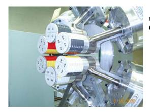
miniSeGA: A barrel of six close packed detectors (Inner diameter ~10.2 cm).
