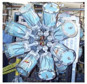
betaSeGA: 16 detectors in 2 rings surrounding beam line in a diameter of 17.3cm.
