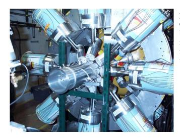
plungerSeGA: two rings of 8 detectors each at maximum forward (30°) and backward (140°) angle in order to obtain maximum Doppler shift of gamma lines for lifetime measurement in RDDS technique.
