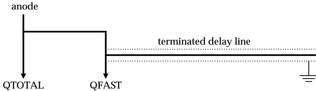
Figure 46 - A simple schematic of the method of producing the PSD signal.
