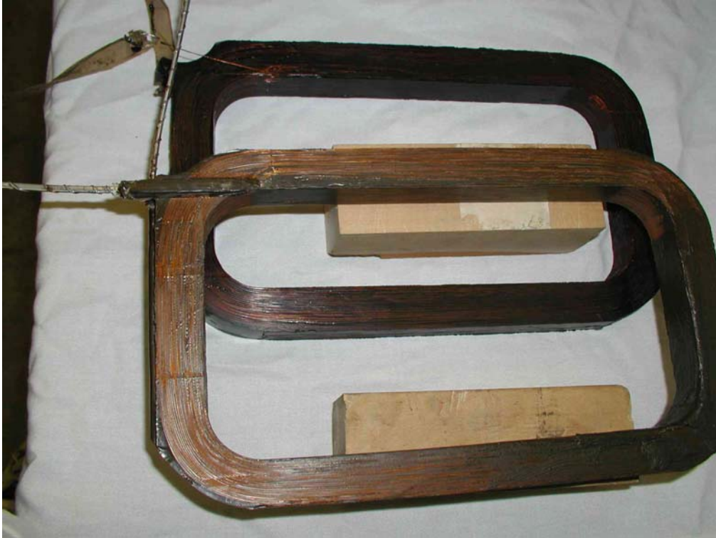
Fig. 2-2: Examples of a Stycast® epoxy-potted coil (in back) and a CTD-422 cyanate-ester-potted coil (in front).
