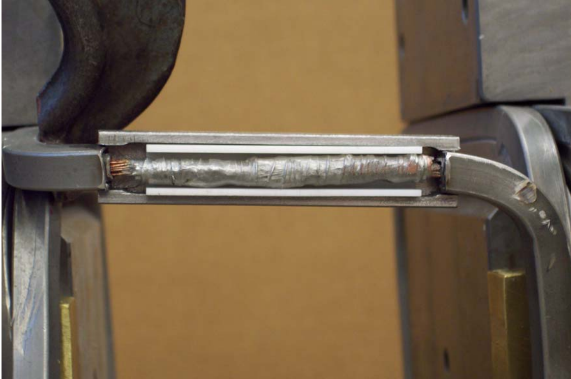
Fig. 3-7: The joint that connects the coils in series is comprised of the solder wire bundle surrounded by two clamshell halves made of an outer stainless steel jacket with a Macor® insert to prevent the conductor from making contact with ground. Seen here is a cutaway: one of the two clamshell halves.
