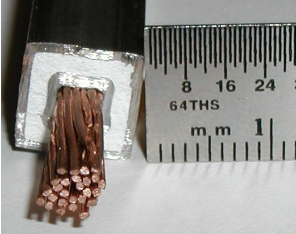
Fig. 1-2: Metal oxide insulated cable-in-conduit conductor. The outer and inner conduits are 316 stainless steel, about 1 mm thick each. The white layer is MgO and is about 2 mm thick. The entire cross section is 1 cm x 1 cm. The inner conduit contains strands of copper/NbTi.
