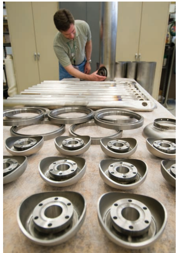
Finished niobium and titanium components for assembly into superconducting cavities for the NSCL reaccelerator; NSCL engineer Patrick Glennon is pictured in the background.
