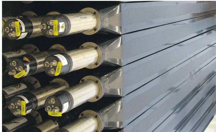
Figure 1 Picture of MoNA bars without cabling
